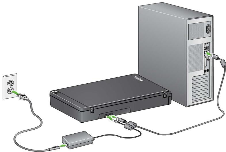
5. Connect the other end of the USB cable to an open USB port on your PC.
